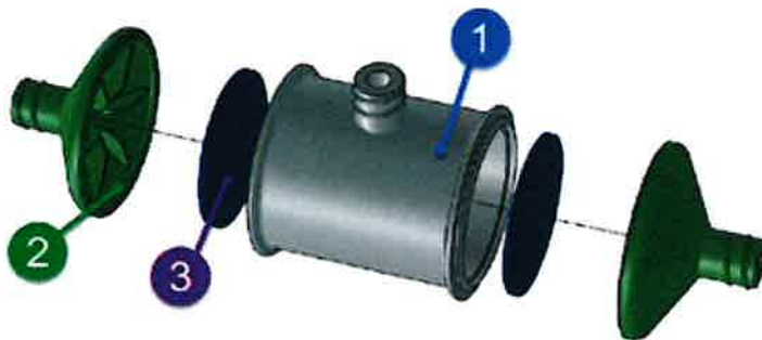
Figure 1. ClearPlasma™ device (1) body, (2) cup, (3) membrane
