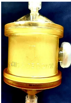
Figure 3: Flow direction marked on the device an arrow “This side down”
