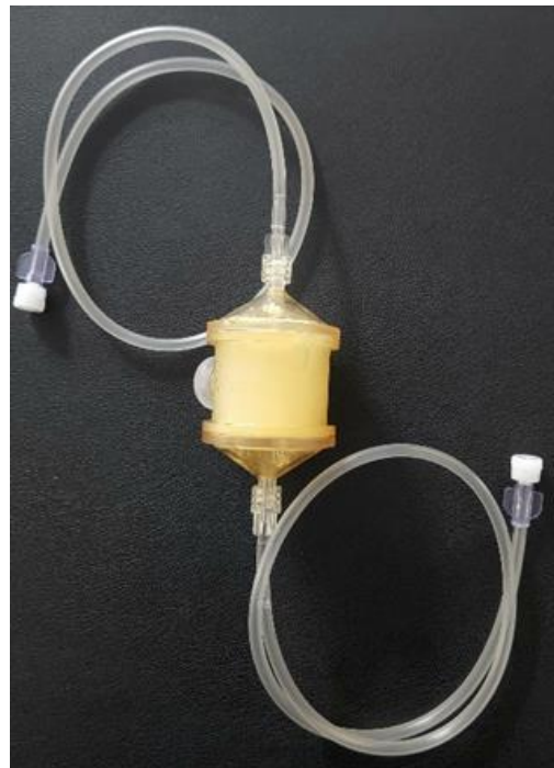
Figure 1: ClearPlasma™ device (1) body, (2) cup, (3) membrane Figure 2: ClearPlasma™ device and its components – as provided to the user.
